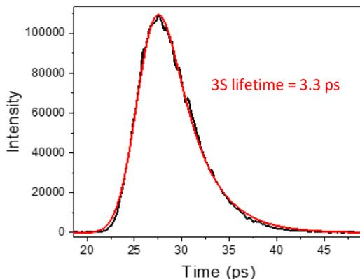
Fig. 1. Example of time-resolved SHG signal, here resonant for the 3S exciton state in Cu<sub>2</sub>O.
